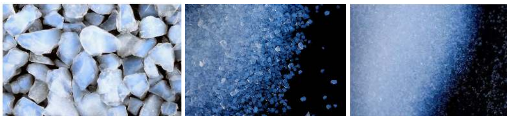
Figure 1. Images of Kwark ® brand silica aerogel granulates and powders produced by Enersens. Right to left: detail of mm-sized aerogel granules; Kwark ® GS granulate; Kwark ® XP500 powder.
