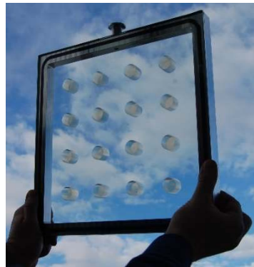
Figure 1: Prototype of vacuum glazing with transparent silica aerogel pillars.
