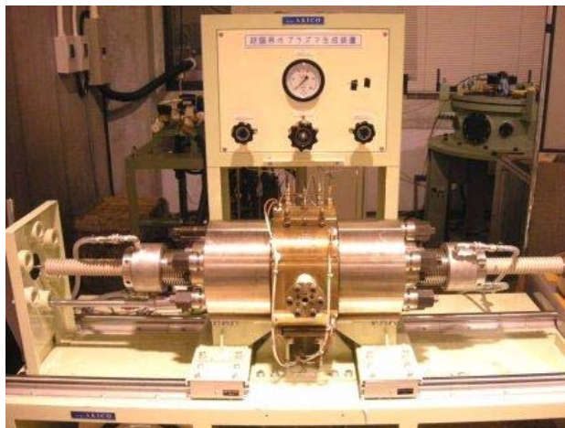
Fig. 2. Photograph of the experimental apparatus for sub-critical water reactor with plasma discharge.
