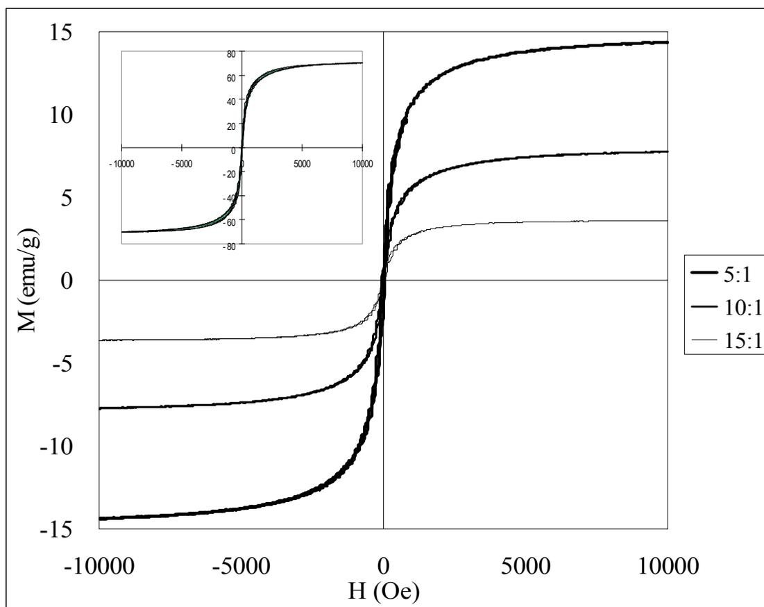
**Figure 3 Magnetization curve of magnetic nanocomposites with different polymer:SPIONs mass ratio: 5:1; 10:1;15:1. Experimental conditions: 160 bar, 15°C, polymer concentration 7.5 mg/mL, nozzle size 175  $\mu$ m. The insert is the normalized magnetization based on the SPIONs weight percentage.**
