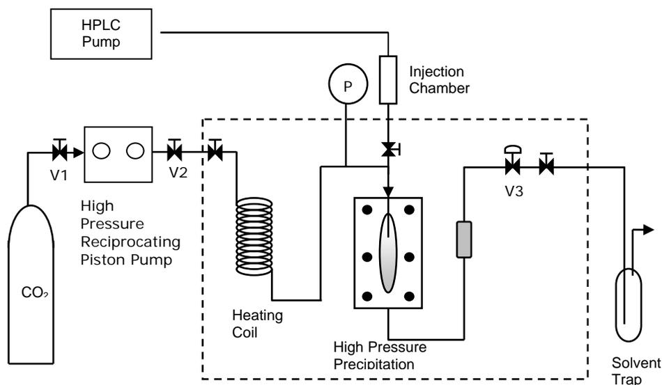
Figure 1 Schematic diagram of the ASES apparatus.
