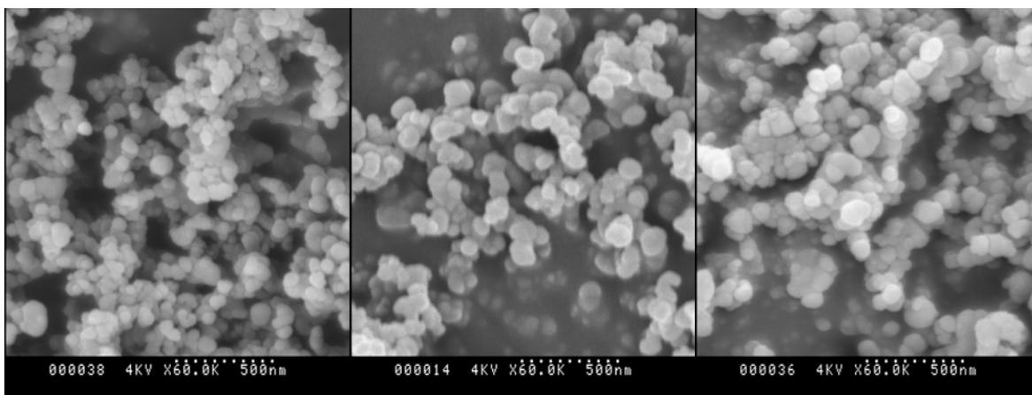
**Figure 2** Eudragit-SPION nanocomposite produced by ASES from polymer solutions of (left) 5 mg/mL, (middle) 7.5 mg/mL, (right) 10 mg/mL. Experimental conditions: 160 bar, 15°C, polymer: SPIONs mass ratio 10: 1.
