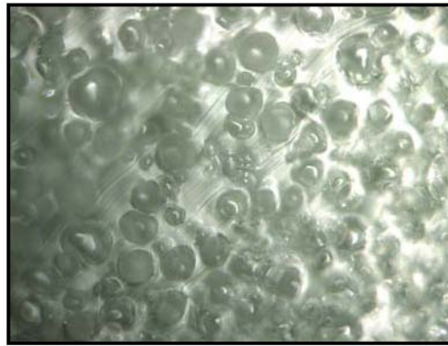
Figure 1: Foamed injection molded part
