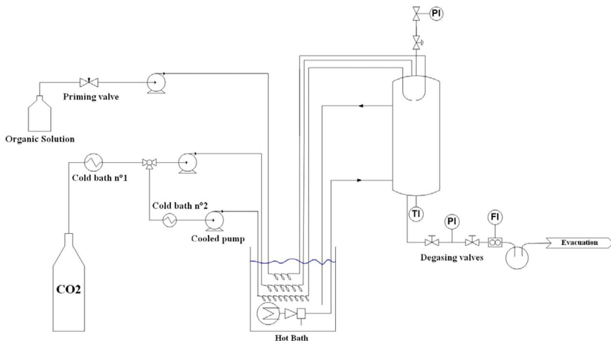
**Figure 1** Experimental device
