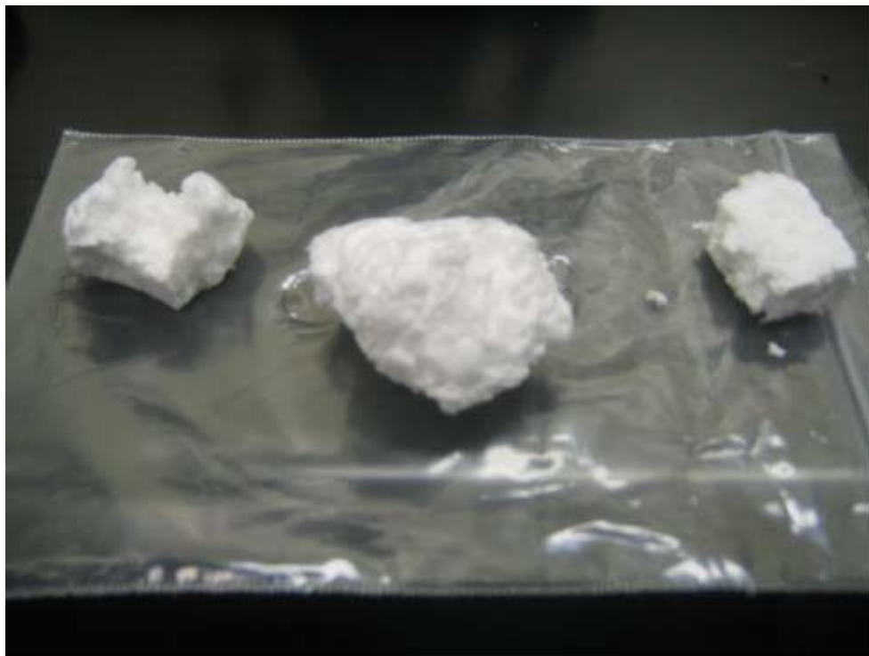
Figure 3: Unloaded SIBS polymer samples (L-Front; Center and R-Back) exposed with SC- \text{CO}_2 at P = 28 \text{ Pa} and T = 318 \text{ K} for an equilibrium time of 86400 s.
