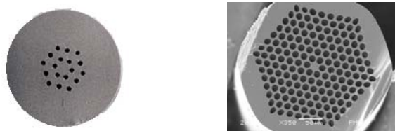
Figure 1. SEM photos of the ends of different “holey” fibres. In this paper, we have used fibre on the left which has 18 holes each 5 microns in diameter.
