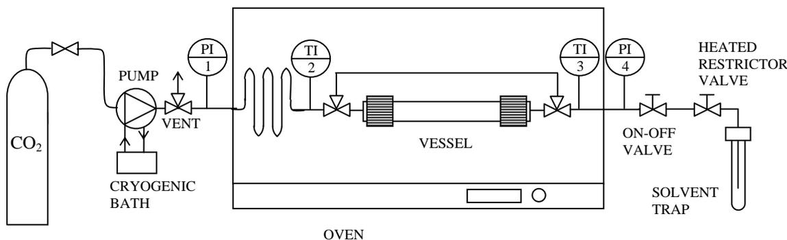
Fig. 2. Experimental apparatus.
