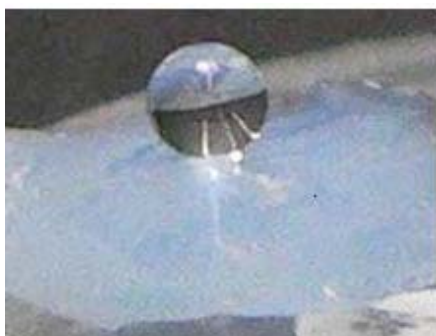
Figure 1. Piece of aerogel with 60% of TRIMOS with a water droplet on the top.
