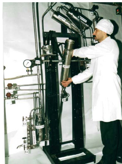
Fig. 2. Pilot setup with natural circulation of CO 2 ( V_{\text{extractor}} 5 \text{ l} )
