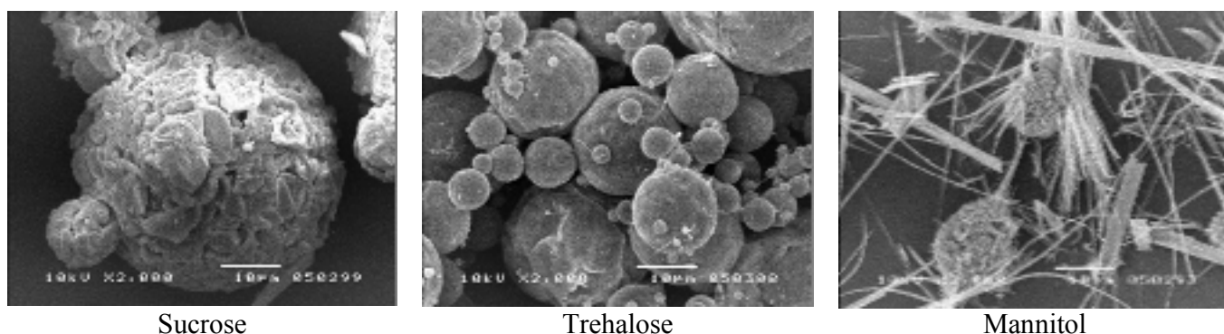
Figure 2 SEM pictures of particles produced from saturated solutions
