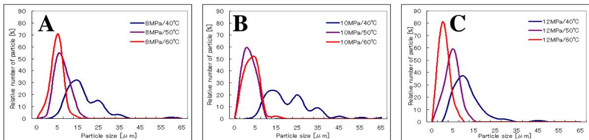
**Figure 4.** Particle size distribution of the processed  $\beta$ -carotene particles precipitated from at various conditions. (A) 8 MPa, 40-60 °C; (B) 10 MPa, 40-60 °C; (C) 12 MPa, 40-60 °C;
