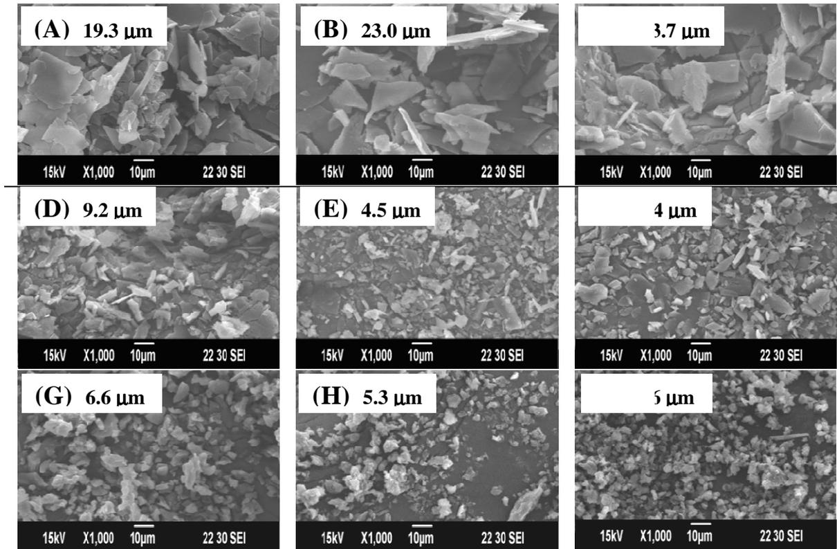
**Figure 3.** SEM image (1000x magnification) of the processed  $\beta$ -carotene particles precipitated from 5 mg/mL  $\beta$ -carotene-DCM solution at various conditions. (A) 8 MPa, 40°C; (B) 10 MPa, 40°C; (C) 12 MPa, 40°C; (D) 8 MPa, 50°C; (E) 10 MPa, 50°C; (F) 12 MPa, 50°C; (G) 8 MPa, 60°C; (H) 10 MPa, 60°C; (I) 12 MPa, 60°C;
