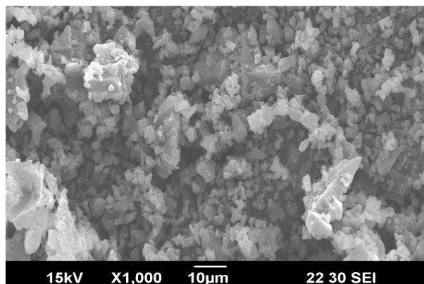
**Figure 1: SEM image of original  $\beta$ -carotene particles (1000x magnification)**
