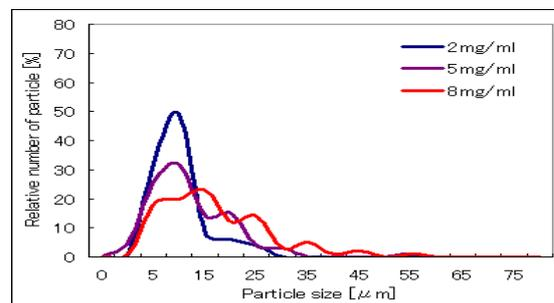
**Figure 6.** Particle size distribution of the processed  $\beta$ -carotene particles precipitated from at 8 MPa, 40 °C, 2-8 mg/mL;
