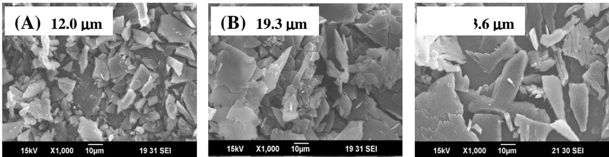
**Figure 5.** SEM image (1000x magnification) of the processed  $\beta$ -carotene particles precipitated from  $\beta$ -carotene-DCM solution at various conditions.
