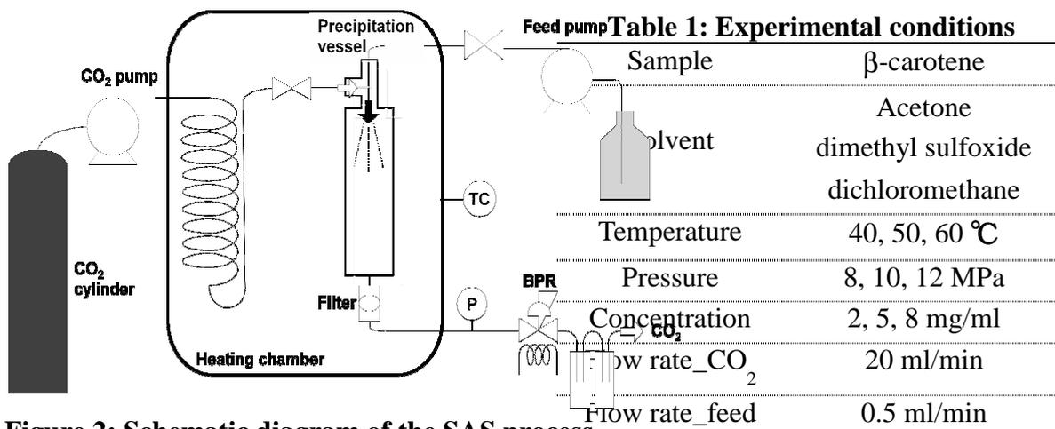
Figure 2: Schematic diagram of the SAS process
