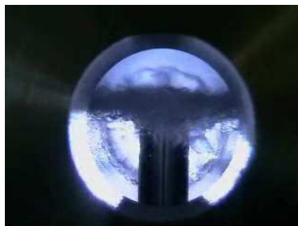
Figure 4: Ultrasound sonotrode acting in two phasic pure carbon dioxide at ambient temperature [13]
