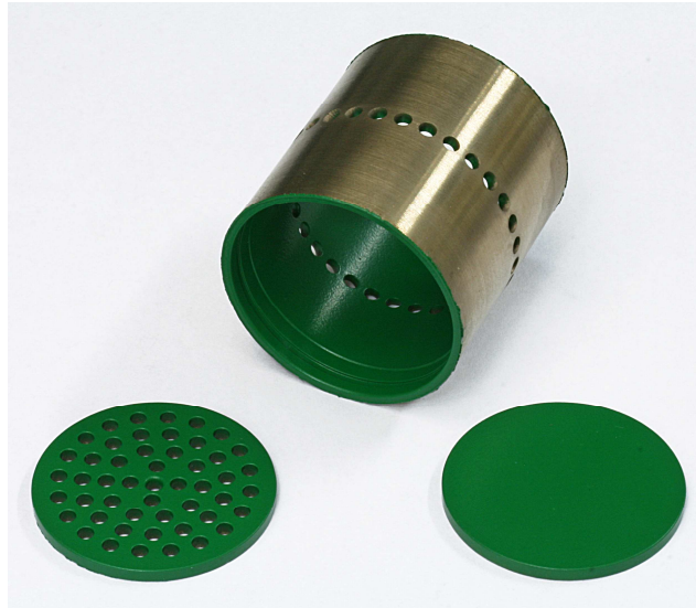
Figure 3 : Cylindrical shaped porous mould used for foaming
