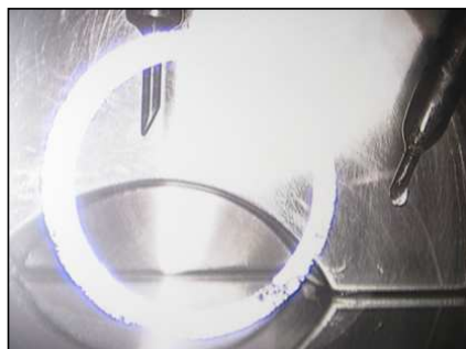
Figure 7: Droplet formation on diagonal capillary with no droplet on vertical capillary
