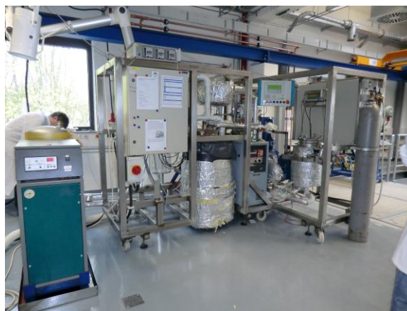
Fig 2. PGSS-drying plant at BOCHUM
