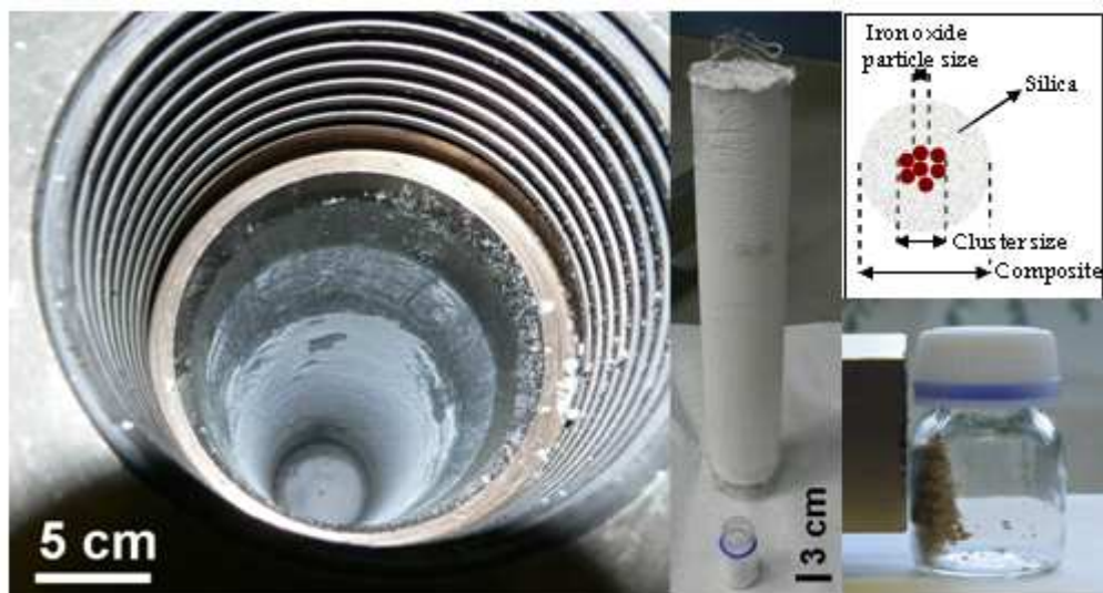
Figure 1. Photographs of the supercritical reactor (left image) and the Pyrex vessel (with glass wool cover; middle image) just after an experiment of pure silica particles. The collected powder can be seen in the lower part of the middle image. A typical batch yielded 2 grams of material. Right upper image presents a schematic view of the magnetic responsive core-shell nanospheres which are also shown in the lower panel.
