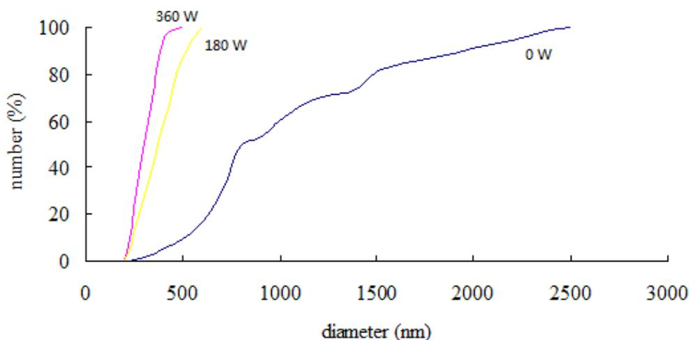
Figure 4 The particle size distribution of PEG-PLA particles prepared with different ultrasound power
