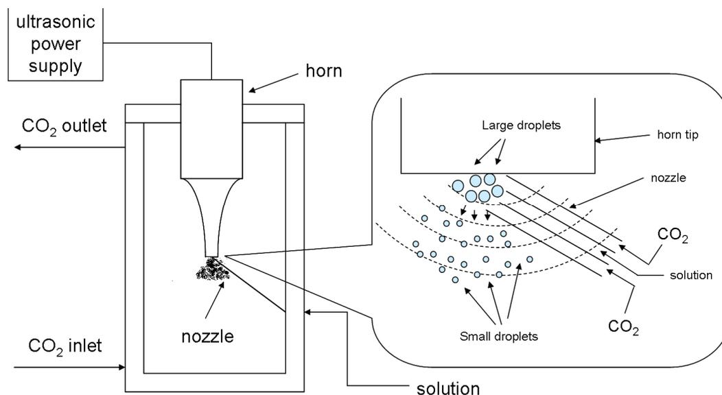
**Figure 2** The diagram of the formation of droplets in the SEDS-EM process
