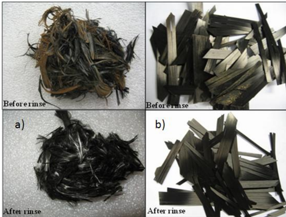
Figure 2: pictures of fibers in different conditions before and after rinsing, a) subcritical, typical aspect after an efficient resin solvolysis b)supercritical
