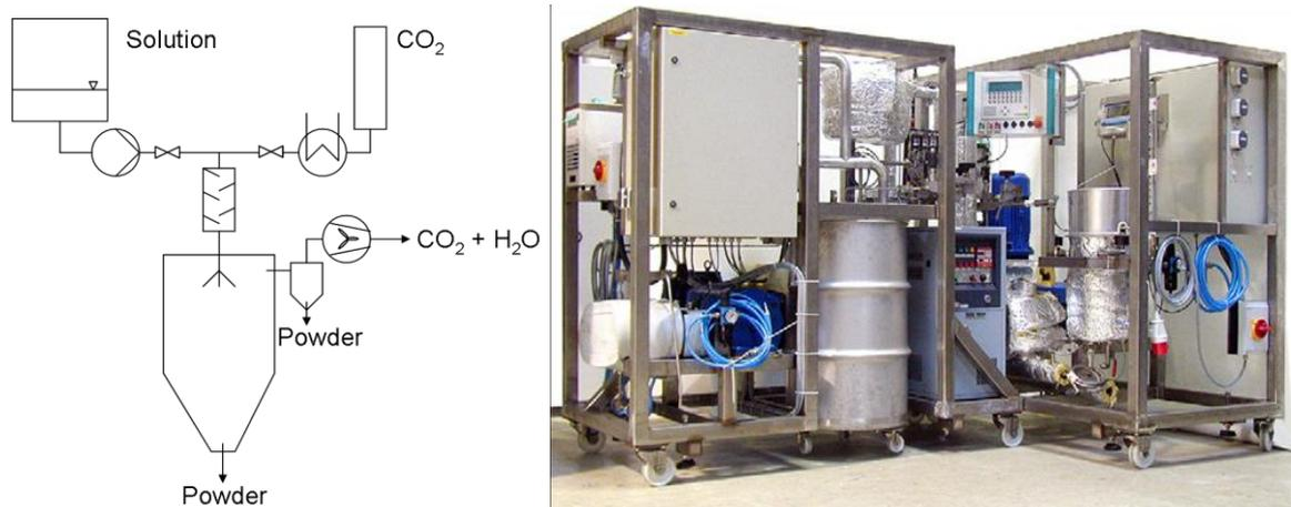
**Figure 1:** Schematic diagram and picture of the PGSS- drying pilot plant
