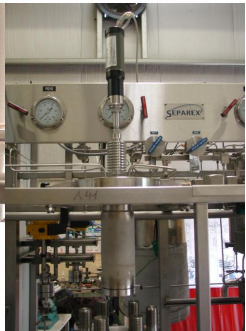
Figure 3: High-pressure (500 bar) high-temperature (450°C) Stirred Reactor for particle design Figure 4: Safe particle harvesting
