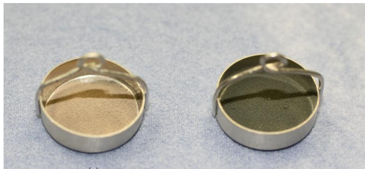
Fig. 3 Photograph of samples (a) before and (b) after chlorination.
