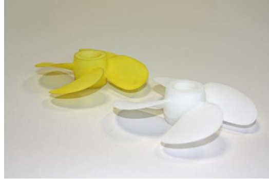
Figure 11: High pressure colored laser-sinter body before and after impregnation with yellow dye
