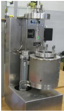
Figure 2: High pressure vessel with 1.5 L, 200 bar, 300 °C
