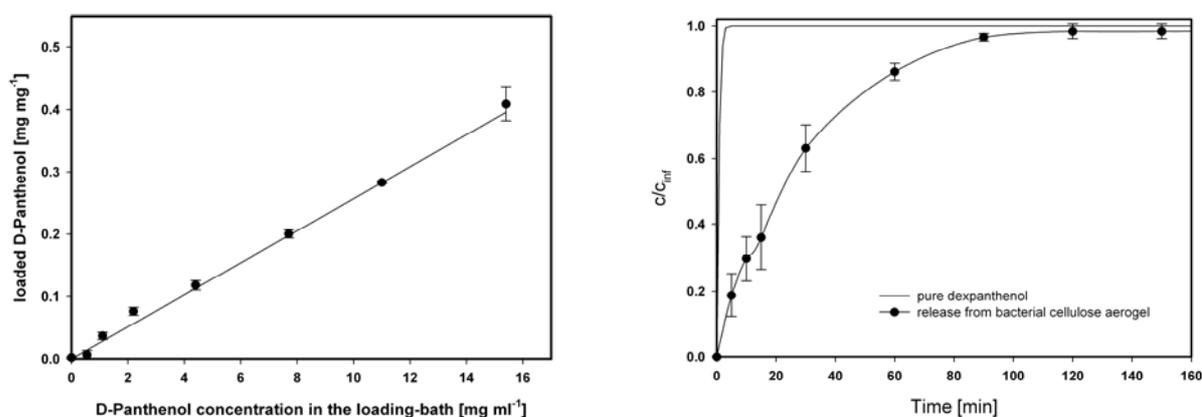
**Figure 4:** loading isotherm for the loading of D-panthenol (dexpantenol) onto bacterial cellulose matrices (left), and comparison of the dissolution of pure D-panthenol and D-panthenol loaded onto a bacterial cellulose aerogel (right)
