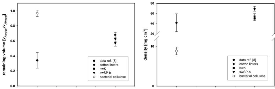
**Figure 1:** Remaining volumes (left) and densities of aerogels (right) obtained from commercial pulps and bacterial cellulose in dependence of the solid content for alcogel
