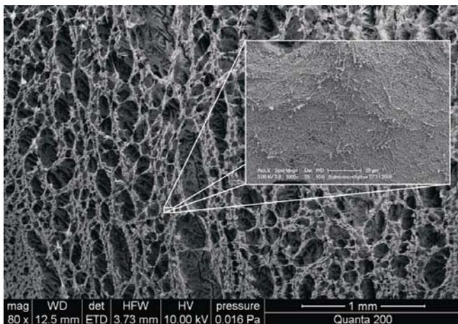
**Figure 3:** SEM-images of the macro- and microporous domains of a bacterial cellulose aerogel.
