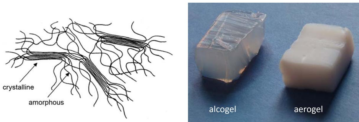
Figure 2: Fringed-micelle model of polymer crystallinity (left). Bacterial cellulose alcogel prior to and after  $scCO_2$  drying (right).
