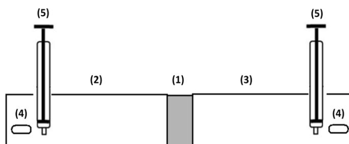
**Figure 4:** Schematic representation of the dynamic assay apparatus. (1) – Scaffold sample; (2) – feed chamber; (3) –permeated chamber; (4) magnetic stirrer; (5) – syringe for sampling.
