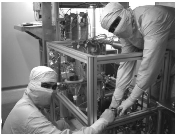
Figure 1: GMP version of CAN-BD installed at Serum Institute of India (Pune, India) for production of myo-inositol based inhalable dry powder measles vaccine for NHP toxicity study and Phase I clinical trials.
