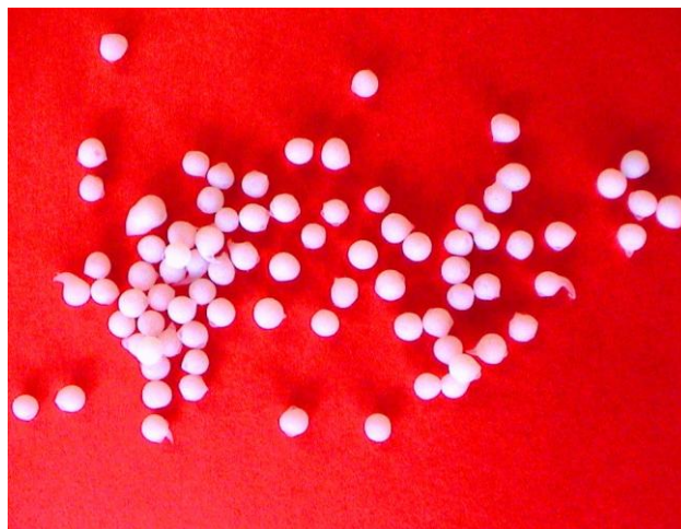
Figure 1: Alginate aerogels obtained by ionic cross-linking using ionic diffusion method.
