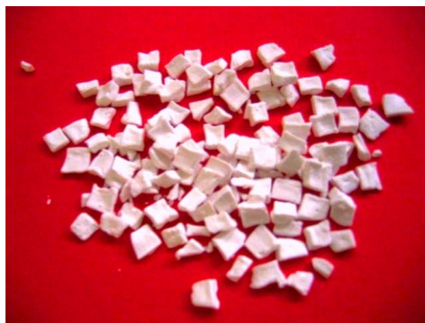
Figure 2: Alginate aerogels obtained by ionic cross-linking by the internal setting method using chelator and initiator.
