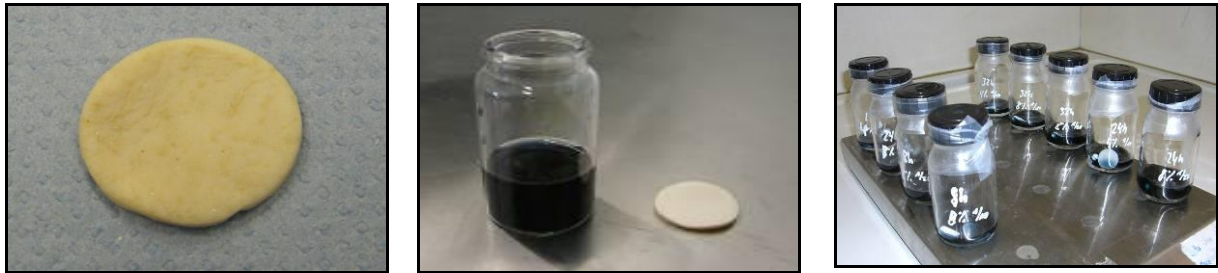
Figure 1: Skin ( \text{Ø} 2 cm), ratio solution to skin, tanning glasses
