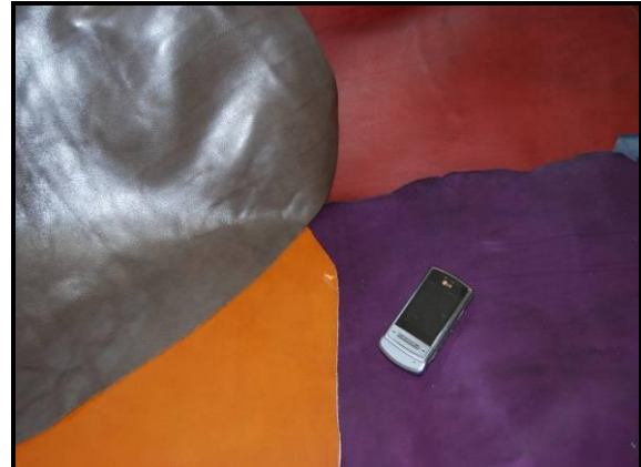
Figure 8: Examples for high pressure Cr tanned leathers
