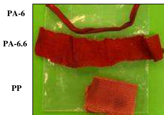
Figure 6: Sc-CO 2 dyeing results obtained with optimized parameters: P=200bar; QCO 2 =3g/min; 5% Milli-Q H 2 O; 10% dye (w/w).
