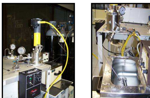
Figure 3: Supercritical fluid Thar R100 system with an auxiliary SFE cell as the dyeing vessel employed in analytical scale tests.
