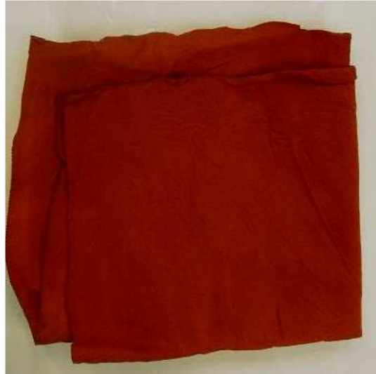
Figure 7: SC-CO 2 dyeing results obtained for PA-6.6 samples with 70cmx30cm size in the scaled-up process.
