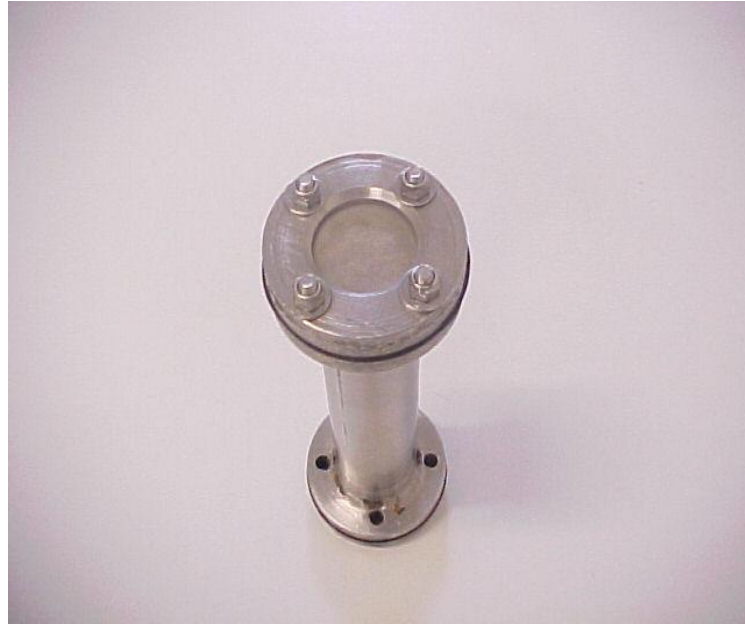
Photography 1: Stainless steel cylinder of 22 cm 3 .
