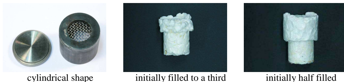
Figure 5: Foaming of Biograde 220C
