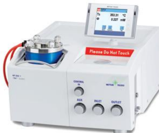
Figure 2: HP DSC1 STAREe, METTLER TOLEDO apparatus.
