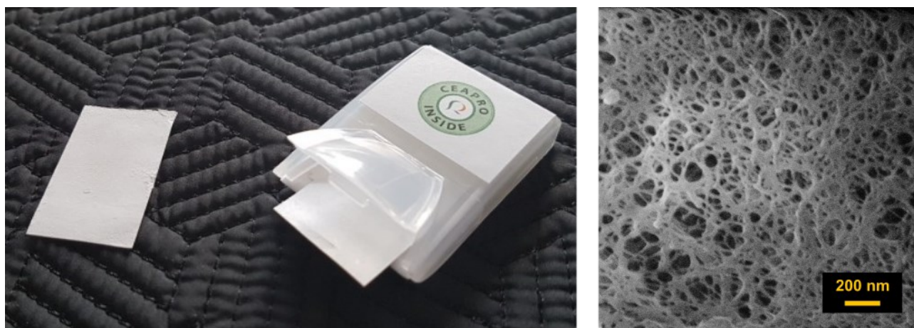
Figure 3. Fast dissolving strips (size 2x3 cm) made from PGX Sodium Alginate aerogel, the specific surface area of the strips is tunable ranging from about 100 to 200 m 2 /gram - shown strip has 5 m 2 - (left). The open-porous structure is maintained in the strip (right).
