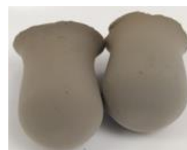
Figure 1. Macroscopic picture of the recovered ZIF-8@GO / PEI aerogel.
