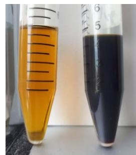
Figure 1. picture of the 100g/l SFE extract (left) and 100 g/l Soxhlet extract (right)
