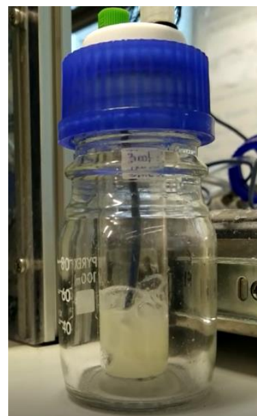
Figure 1. Bubbling process to trap flavoring compounds into food trapping material
