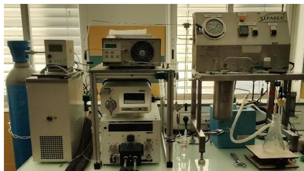
Figure 1. Sc-CO 2 apparatus (lab-scale)
