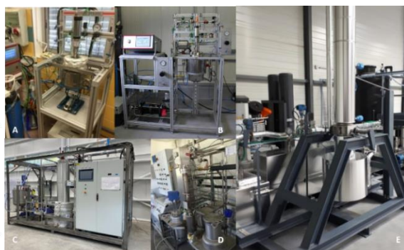
Figure 1. Multi-scale equipment: A-200mL batch b , B-1L batch a , C-10 kg/h unit a , D-1 kg/h unit b , E-100 kg/h unit c
