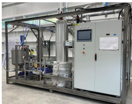
Figure 1 WAO continuous pilot-scale equipment from A3i-Inovertis
