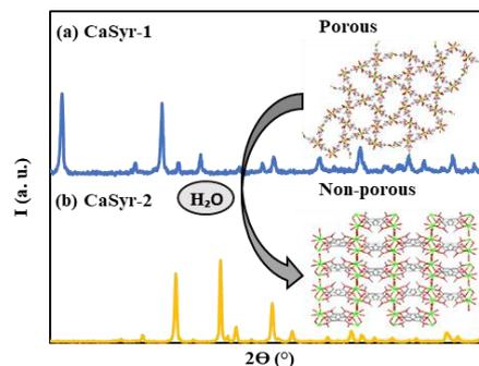
**Figure 1.** XRD pattern of (a) porous and (b) non-porous Ca-Syr, and their crystalline structures (inlets)
