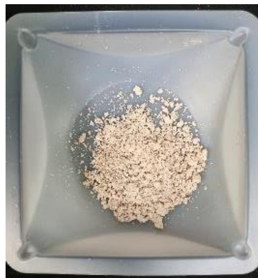
Figure 2. Encapsulated astaxanthin after the SAS process
