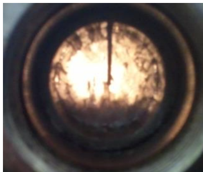
Figure 2: View to high pressure cell for the system of vanillin in argon at a pressure of 150 bar and at a temperature of 40°C.
