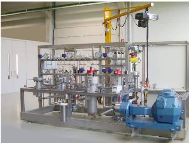
Figure 6: 5 l/1000 bar research unit (NATEX)
