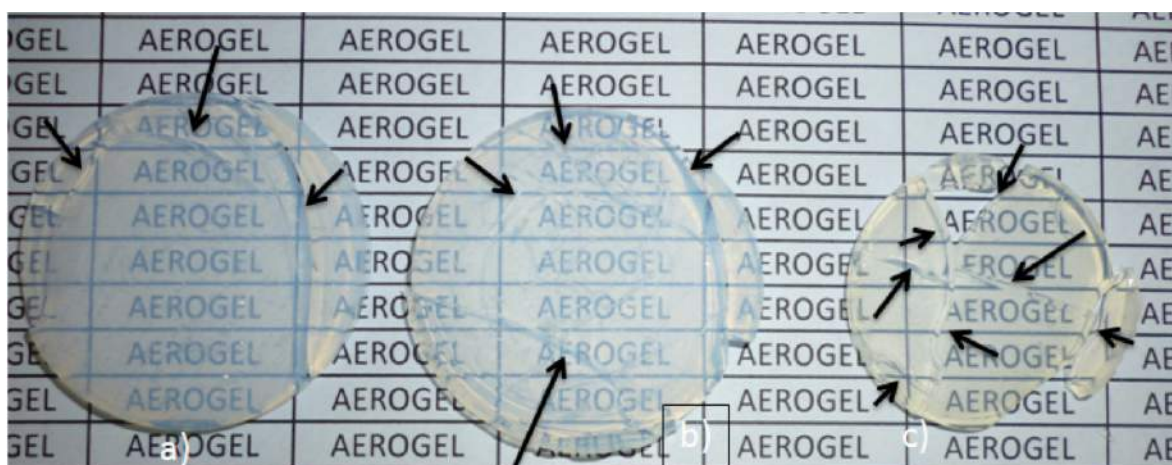
Figure 1. Aerogel monoliths obtained with surface modification treatment and solvent pre-treatment with a) Hexane, b) Heptane; and c) Acetone.
