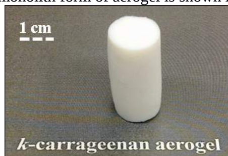
Figure 3: Image showing the monolith form of k -carrageenan aerogel (3 wt %).
