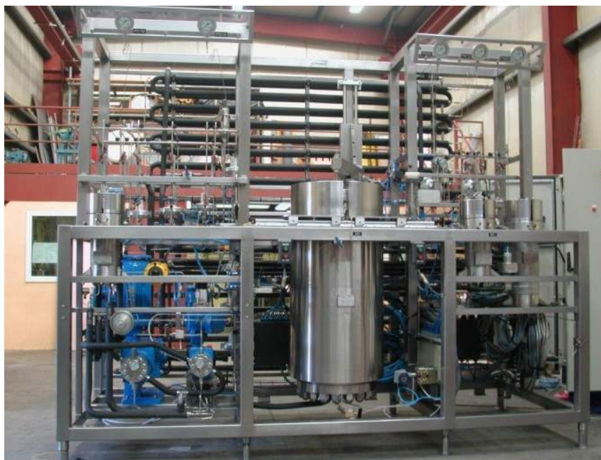
Figure 5: Semi-industrial 170-litre SFD Unit
