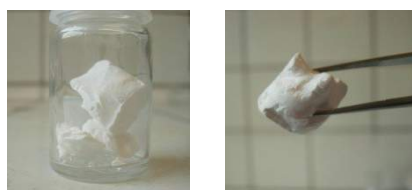
Figure 3: Pictures of an aerogel obtained from an organogel of gelator 1 1 wt% in toluene
