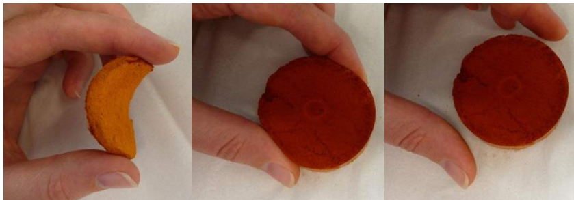
Figure 4: Flexible RF-Aerogel produced with R/W molar ratio 0.006-0.008
