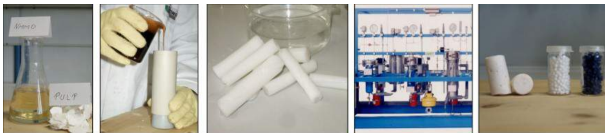
Figure 2: Starting material: pulp and 50 % NMMO solution – shaping – regenerated cellulose hydrogels – supercritical drying – Cellulose Aerogels. (Final published report EC project Aerocell 505888-1).
