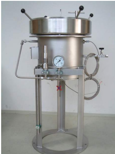
Figure 9: Pilot Plant for Aerocell drying.
