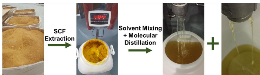
Fig.3 Tobacco Oil Producing Process
