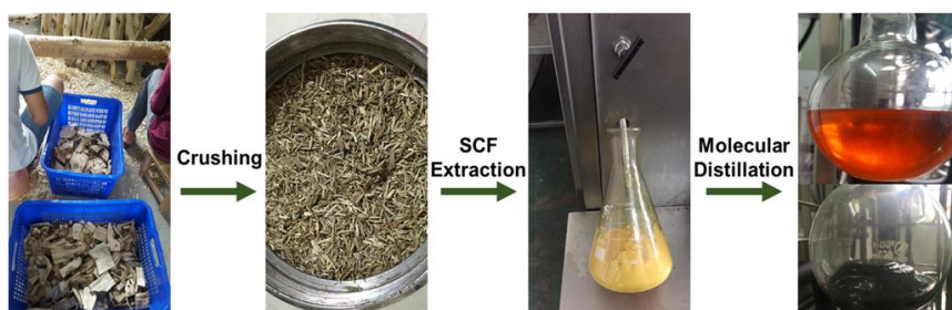
Fig.2 Agarwood Oil Extraction and Separation Combined Process
