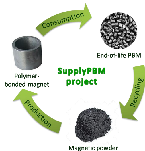
Figure 1: Circular economy route for rare earth polymer-bonded magnets in the frame of SupplyPBM project
