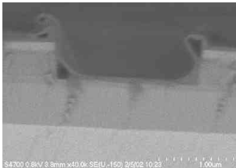
Fig. 5 Swelling and delaminating of polymer film in a trench of a semiconductor wafer induced by SC-CO 2 .
