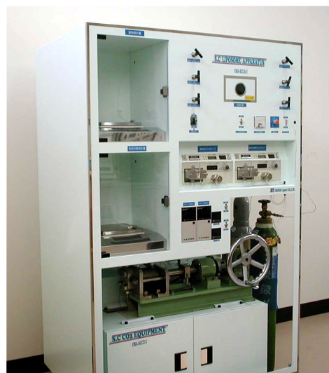
Figure 8. Outlook of the semi batch type liposome production apparatus.
