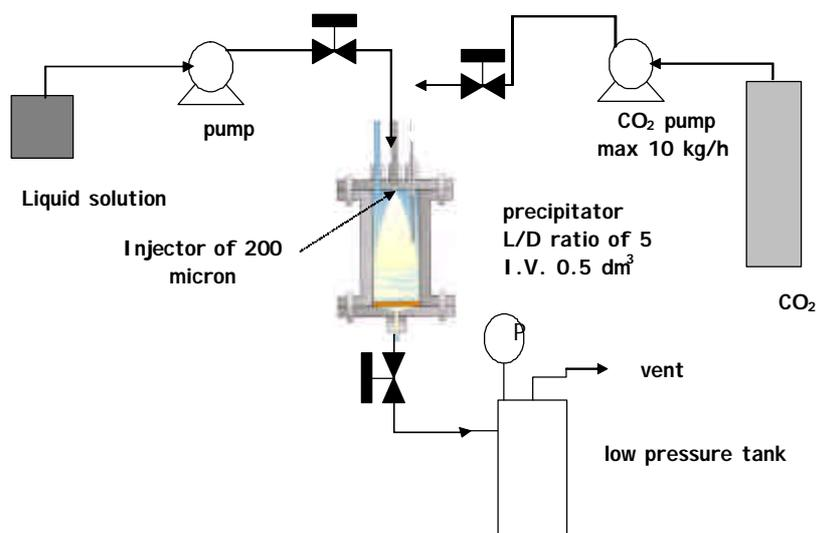
**fig. 1.** SAS laboratory apparatus
