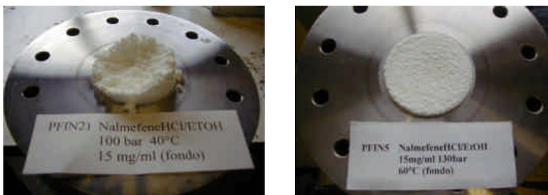
**fig. 3.** Images of the bottom of the Precipitation Vessel.
