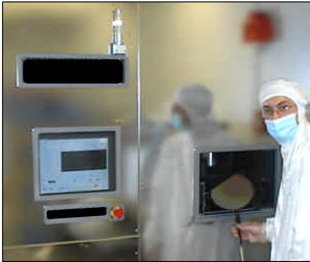
Figure 3: Wafer loading in the chamber
